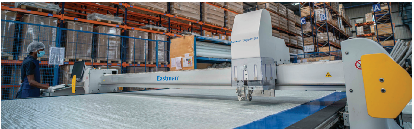
Automated Glass Fabric Cutting Machine, ensures nesting and reduces wastage consistently
